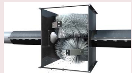
Brush box cleaning
