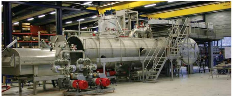
and better natural potato taste. To meet with the industrial requirement of capacities the Multi Stage Vacuum Fryer is developed for a capacity of 1500 kg/hr finished product.
